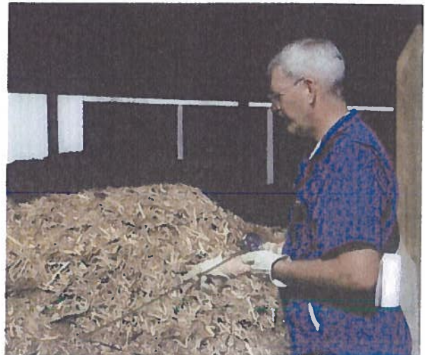
Figure 4. Checking internal temperatures with a composting thermometer is a quick way to determine if moisture and other conditions are suitable for rapid decay and pathogen reduction. (Photo by Tom Glanville, Iowa State University.)
